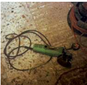
Cable damage covered with tape
